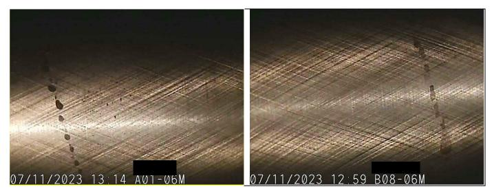
In B9, at the 12:00 bottom position there is a fresh looking mark, possibly some debris has been trapped in the piston ring and has created this score during the barring, hence the non-linear nature of the score as the piston ring has rotated slightly.
