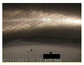
In a number of cylinders evidence of a historic water marks were seen, possibly from the engine being stored for an extended period of time and water collected on the piston crown and between the piston ring and liner. Typical photos are shown below. These are shown for completeness and are unlikely to be associated with the engine derating issues.
