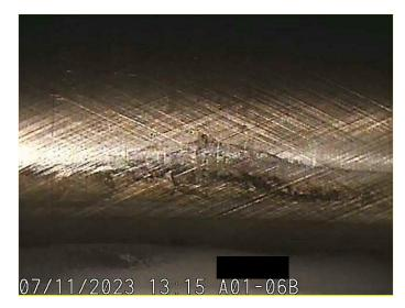
In B10 there is evidence of corrosion pitting, as shown below.
