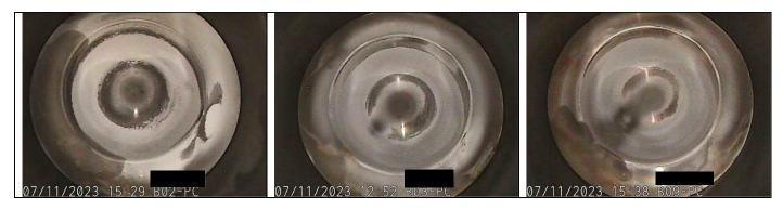
Time constraints limited the number of valves that were inspected and only exhaust valves were seen. Those were similar in condition with light even coating of ash and the seats in good condition.
