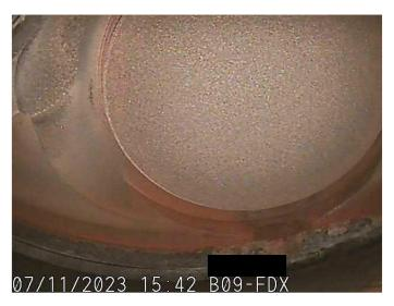
The ash was generally light and even with the exception of B2, B3 and B9 which had patchy ash coverage and exposed areas of piston material.
